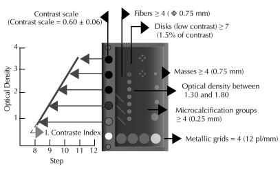
Figure 1. A. Mammographic phantom; B. Image of the breast phantom produced in the mammography services.
