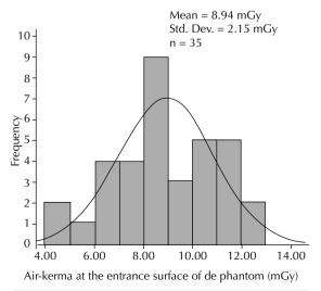
**Figure 3.** Radiation dose at the entrance surface of the phantom (air-kerma) at the mammography services. Goiás, Central-Western Brazil, 2009.
